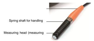
The sensor is to be grasped at the lower shaft segment and is only lightly pressed onto the test object.
