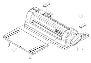
fig. 4 Installation without a spindle
