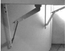
Do block the safety notches in their seats by pushing the table downward. Support locks must remain upright once entered into their seats.
