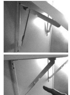
To close the table lift it from the open position, manually help the rails to close by following through the table downward.
