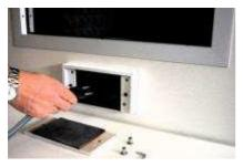
2) Run the cables of the devices which are necessary such as headphones or anything else through the center hole.
