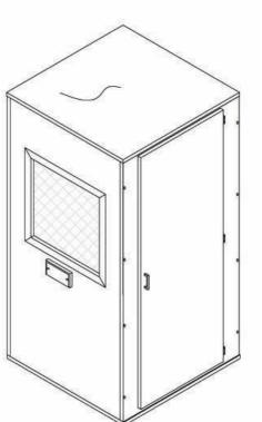
Once performed that, apply stickers signals as follows :put the symbols "MIND THE STEP" and "PUSH" at eye level on the inside part of the door . Apply the yellow and black stripe on the step.
